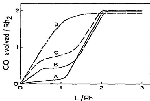
Fig. 2. Carbon monoxide evolution on addition of  $\text{PMe}_2\text{Ph(L)}$  to  $\text{Rh}_2\text{Cl}_2(\text{CO})_4$  in cyclohexane solution. A. Under CO (1 atm) at  $20^\circ\text{C}$ . B. Under  $\text{N}_2$  (1 atm) (25 ml) at  $20^\circ\text{C}$ . C. Under  $\text{N}_2$  (1 atm) (75 ml) at  $20^\circ\text{C}$ . D. Under  $\text{N}_2$  (1 atm) (75 ml) in refluxing solution ( $81^\circ\text{C}$ ).
