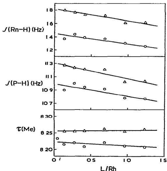
Fig. 5. Graphs showing the dependence of  $J(\text{Rh-H})$ ,  $J(\text{P-H})$  and  $\tau$ -value for the  $\text{PMe}_2\text{Ph}$   $^1\text{H}$  NMR signal (sharply resolved double doublet) on addition of  $\text{PMe}_2\text{Ph}$  to  $\text{Rh}_2\text{Cl}_2(\text{CO})_4$  in cyclo- $\text{C}_6\text{D}_{12}$ , saturated with  $\text{N}_2$  ( $\Delta$ ) or  $\text{CO}$  ( $\circ$ ).
