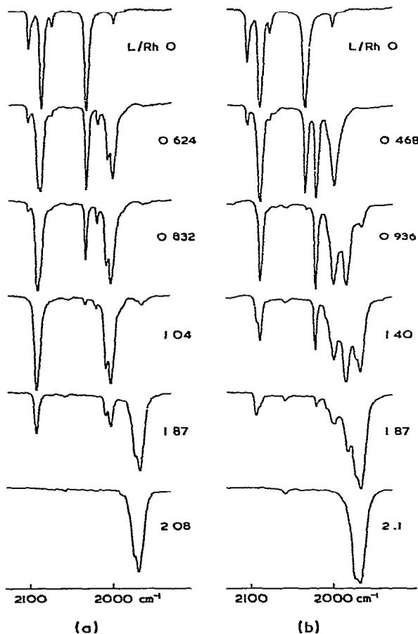
Fig. 1. Infrared spectra of  $\text{Rh}_2\text{Cl}_2(\text{CO})_4$  in cyclohexane on addition of  $\text{PMe}_2\text{Ph}(\text{L})$  either (a) saturated with CO or (b) with  $\text{N}_2$  bubbled through the solution for 10 min after each addition of  $\text{PMe}_2\text{Ph}$ .
