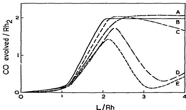
Fig. 3. Carbon monoxide evolution on addition of  $\text{PMe}_2\text{Ph(L)}$  to  $\text{Rh}_2\text{Cl}_2(\text{CO})_4$  in different solvents under an atmosphere of carbon monoxide ( $20^\circ\text{C}$ ). A, toluene; B, cyclohexane; C, methylethylketone (butan-2-one); D, propan-2-ol; E, ethanol.
