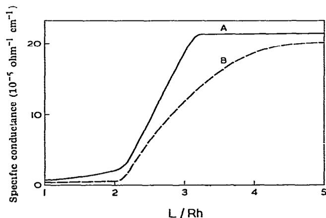
Fig. 4. Specific conductance of a solution of  $\text{Rh}_2\text{Cl}_2(\text{CO})_4$  ( $2 \times 10^{-3} \text{ mol dm}^{-3}$ ) in ethanol on addition of  $\text{PMe}_2\text{Ph}(\text{L})$  with either CO (A) or  $\text{N}_2$  (B) bubbled through the solution ( $20^\circ \text{C}$ ).
